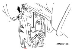
Push the power trim and tilt switch "DN" (down) to lower the outboard motor to the desired position.
