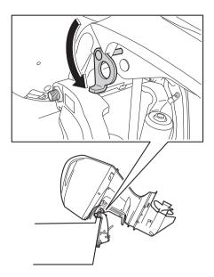
. Once the outboard motor is supported with the tilt support lever, press the power trim and tilt switch "DN" (down) to retract the trim rods. *NOTICE:* Make sure that the trim rods retract completely during mooring. This protects the rods from marine growth and corrosion, which could damage the power trim and tilt mechanism. [ECM00254]
