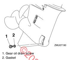
5. Remove the oil level plug and gasket to allow the gear oil to drain completely. *NOTICE:* Check the used gear oil after it has been drained. If the gear oil is milky or contains water or a large amount of metal particles, the gear case may be damaged. Have a Yamaha dealer check and repair the outboard motor. [ECM00714]
