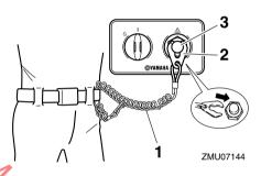
1 Engine shut-off cord (lanyard) 2. Clip
