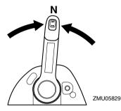
Press the power trim and tilt switch "UP" (up) until the outboard motor has tilted up completely.
