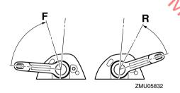
2. After the engine is at idle speed in gear, move the control lever firmly and crisply into the neutral position.
