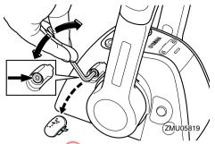
When constant speed is desired, tighten the adjuster to maintain the desired throttle setting.
