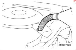
Recommended engine oil: YAMALUBE 4M FC-W or 4-stroke outboard motor oil Engine oil quantity (without oil filter replacement): 6.0 L (6.34 US qt, 5.28 lmp.qt) Engine oil quantity (with oil filter replacement): 6.3 L (6.66 US qt, 5.54 lmp.qt)
