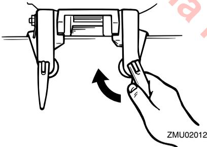
2. If the restraint cable attachment is equipped on your engine, a restraint cable or chain should be used. Attach one end to the restraint cable attachment and the other to a secure mounting point on the boat. Otherwise the engine could be completely lost if it accidentally falls off the transom.
