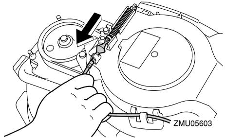
4. Remove the starter/flywheel cover after removing the bolt(s).
