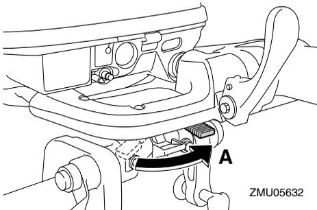
3. Hold the handgrips and steering brackets as shown in the illustration and lift up the outboard motor using two people.
