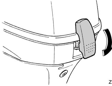
After installing, check the fitting of the top cowling by pushing it with both hands. If the top cowling is loose, have it repaired by your Yamaha dealer.
