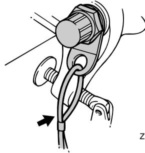
3. Secure the clamp bracket to the transom using the bolts provided with the outboard (if packed). For details, consult your Yamaha dealer. **WARNING! Avoid using bolts, nuts or washers other than those contained in the engine packaging. If used, they must be of at least the same quality of material and strength and must be tightened securely. After tightening, test run the engine and check their tightness.** [EWM00652]
