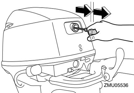
6. After the engine starts, slowly return the manual starter handle to its original position before releasing it.
