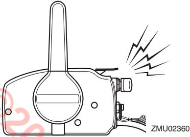
If the alert system has activated, stop the engine as soon as it is safe to do so. Check the oil level and add oil as needed. If the oil level is correct, consult your Yamaha dealer.
