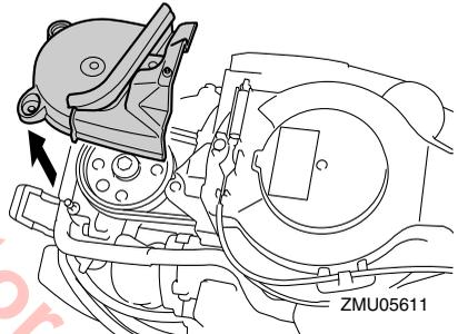
3. Remove the electrical system cover by removing its screw(s).
