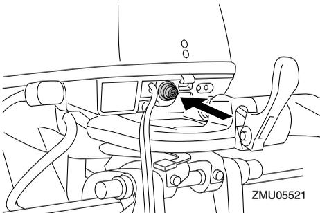
5. Immediately after the engine starts, release the starter button and allow it to re-
